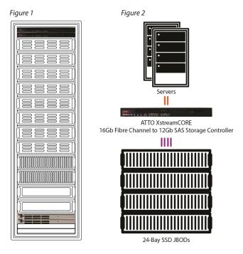
Figure 1 - Dual XstreamCORE bridges with 10 shelves of SSd/ HDD storage connected to a server via 32Gb Fibre Channel
