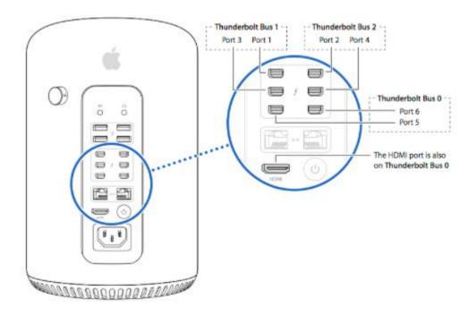
Figure 1. Image via Apple KB article HT202801 Each of the 3 Thunderbolt 2 busses in the Apple Mac Pro have a dedicated bandwidth of 5 Gigabytes per second from the system's PCIe controller.
