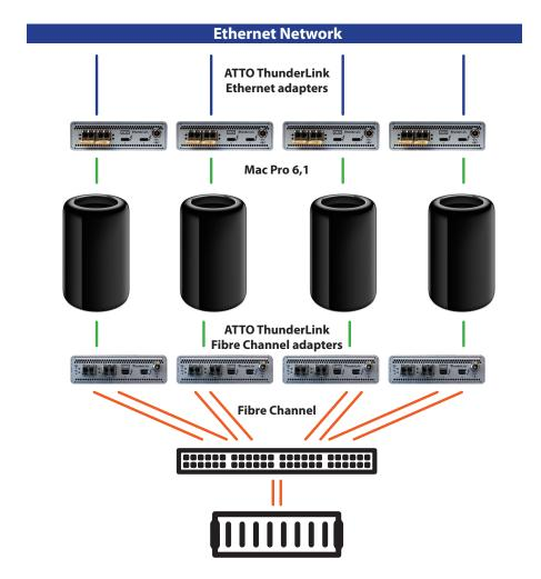
Now virtualize your Mac Pro hosts with ESXi and use ATTO ThunderLink® Thunderbolt™ adapters to efficiently connect to Fibre Channel storage by using an ATTO VMware Ready™ VCG approved ESXi driver. ATTO ThunderLink Thunderbolt enabled Fibre Channel adapters are designed as purpose built devices. With a smaller footprint, and less power required, you achieve the same throughput with a singular device compared to other Thunderbolt enabled solutions.
