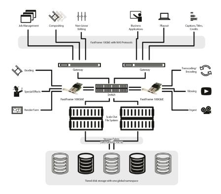
ATTO 25/40/20/100GbE FastFrame NICs in a demanding 4k video environment utilizing NAS storage. This scale-out file system allows shared RDMA access to media storage, with support for one 4K/24fps stream for each workstation using RDMA. Areas in the workflow that don't require real-time uncompressed streaming utilize the gateway to access media files.
