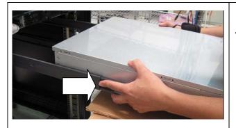
11) Carefully slide bracket pressing lock button to allow CHASSIS SECTION insertion.
