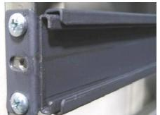
5) INTERMEDIATE SECTION must be inserted into the STATIONARY SECTION before the end bracket is attached. Install bracket to the front cabinet section with 10-32 screws.
