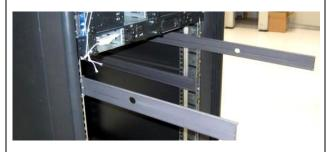
8) Slide out INTERMEDIATE SECTIONS to the lock button.
