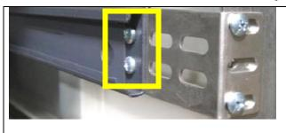
7) Install CHASSIS MOUNTING BRACKET to the rear cabinet section. Screws holding FLANGE MOUNT STATIONARY and CHASSIS MOUNTING BRACKET can be adjust as required. .
