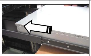
10)Carefully insert CHASSIS SECTION into INTERMEDIATE SECTIONS.
