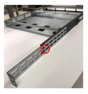
5. To mount (or) remove the Thunderlink (or) XstreamCORE 8100T in the rack, unscrew the lock.
