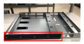
$^{\mbox{Note}}$  The outer rail can be removed from the FlexRack chassis to allow for ease in mounting the rails to the rack.
