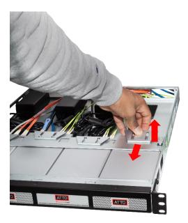
7. Insert the unit from under the rail support as shown in the image below.
