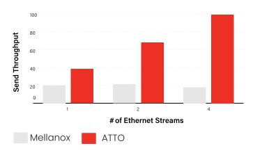
**Test setup:** NIC under test installed in a 2023 Mac Pro M2 Ultra connected to an ATTO Fast Frame N412 installed in a Linux Server running iPerf. MTU = 1500. No tuning.
